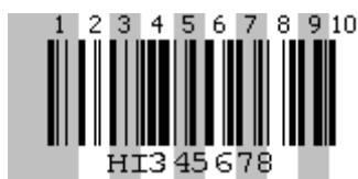
Figure 41: Code 128 Encoding Example
